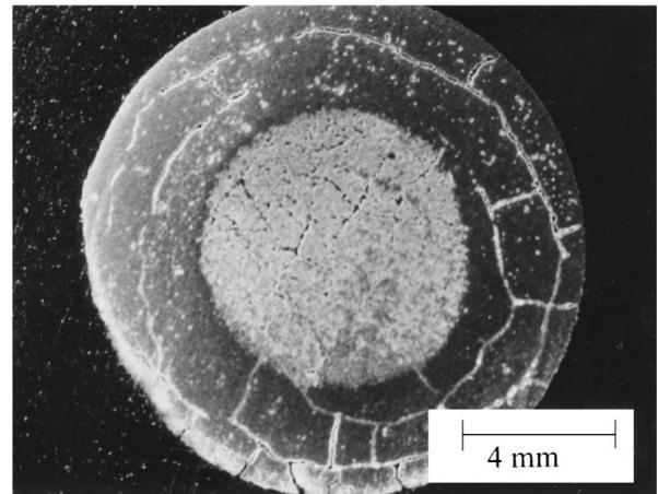
Figure 2 A partially infiltrated  $\text{Cu-NbB}_2$  specimen showing cracking in the infiltrated outer region.
