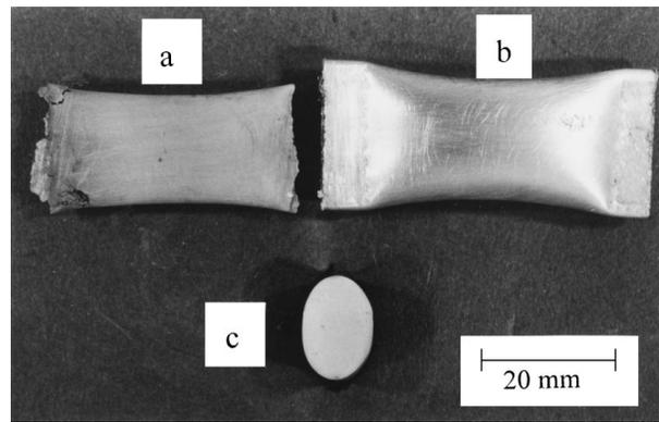
Figure 1 Specimens a) after successful infiltration, b) before heat treatment and c) a cross section through an infiltrated sample.
