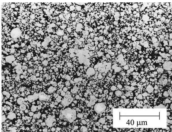
Figure 4 Back-scattered electron image of WC (light) spontaneously infiltrated by Cu (dark).
