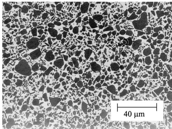
Figure 3 Back-scattered electron image of  $\text{Cr}_3\text{C}_2$  (dark) spontaneously infiltrated by Cu (light).
